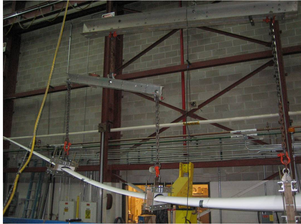
Static Blade Tests for CX-100 (left) and BSDS (right) at the NWTC
