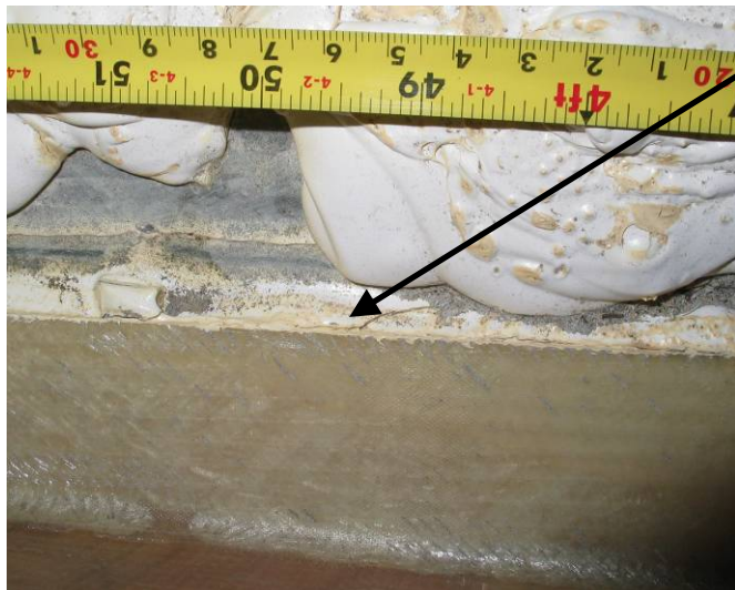
Post-test Photo of CX-100 Shear Web Bond Line at 1200-1300 mm
